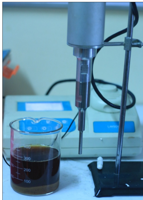
Fig 3: Sonication of the clove powder dissolved in 50 ml water using ultra sonic sonicator (100 W with a titanium horn)
